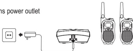
Before using the walkie-talkies for the first time, charge them for at least 14 hours. When the walkie-talkies are connected correctly, the red LEDs light up. The LEDs only signal that the connection is correct and continue to light up even when the battery packs are fully charged.
